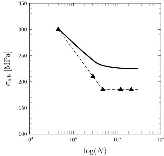
Figure 6. Fatigue strengths of the 34CrNiMo6 steel. The solid line is the model response and the markers denote the experimental data from [5].  $N$  is the number of cycles required for macroscopic crack initiation.
