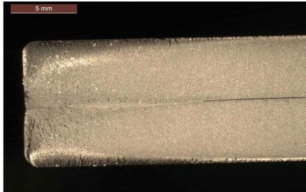
Figure 4. Cracked surface of the fretting specimen.
