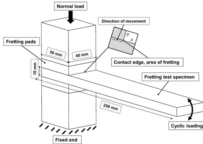
Figure 1. Testing arrangement [5].
