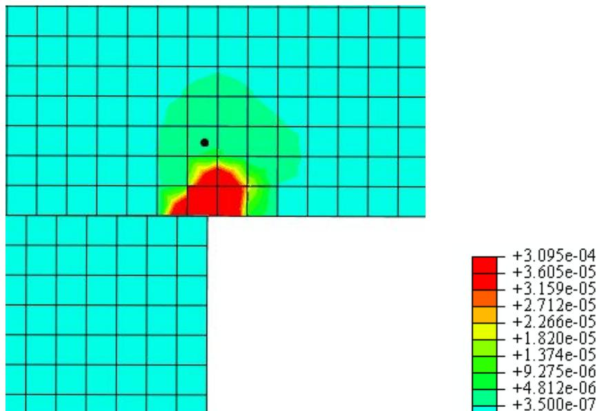
Figure 5. Damage field in the numerical model after 16 cycles at the contact corner point. Maximum value of damage is  $3.1 \cdot 10^{-4}$ . The size of the smallest element is  $5 \mu\text{m}$ .
