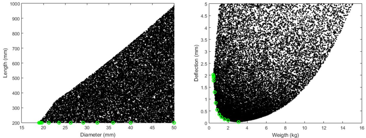
Figure 7. feasible set (dotted area) and the found Pareto optimal set (marked with circles) in design and criterion spaces.
