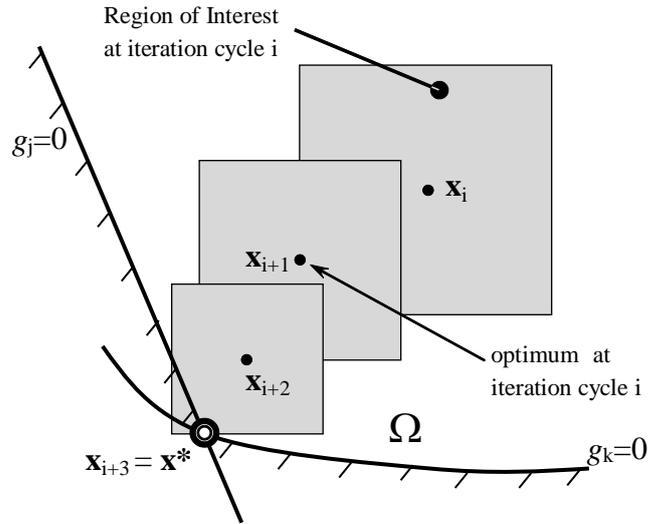
Figure 1. Schematic optimization iteration progress from iteration cycle  $i$  to the optimum  $x^*$ . The size of the region of interest changes during the iteration according to the approximation errors (adaptive ROI) or remains the same (fixed ROI).  $\Omega$  denotes the feasible region.
