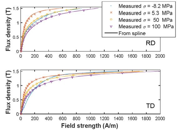
Fig. 2. Comparison of measured and modeled single-valued  $B(H)$  curves of Material 1 in the RD and TD. The measured curves have been obtained by averaging the major hysteresis loop in the  $H$ -direction.
