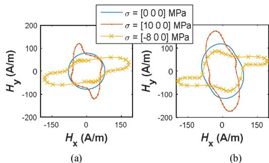
Fig. 5. Field strength loci under different in-plane stress tensors (in notation  $[\sigma_{xx} \sigma_{yy} \sigma_{xy}]$ ) and circular flux density of 1.0 T in Material 1. (a) Isotropic case (only RD parameters used) and (b) anisotropic case.
