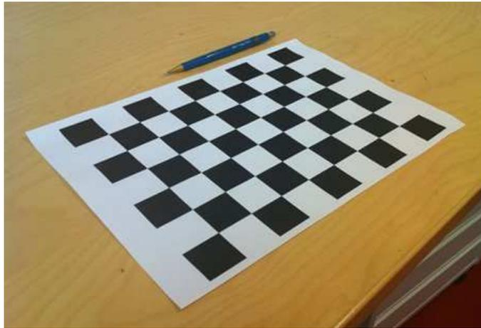
Figure 6: Calibration pattern
